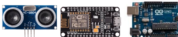
Fig. 4. Main hardware components from left to right side: ultrasound sensor, ESP8266 and arduino Fig. 5.
